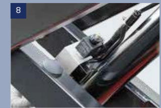
Explosion proof valve: To prevent the machine falling when the oil pipe is leaking
